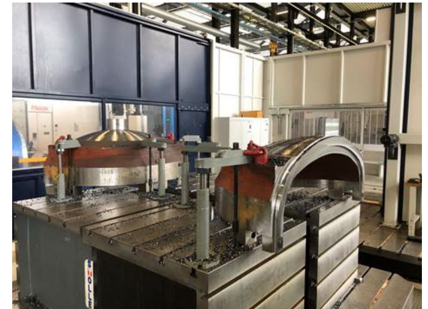
Lower one-half head after HIP and during final machining
