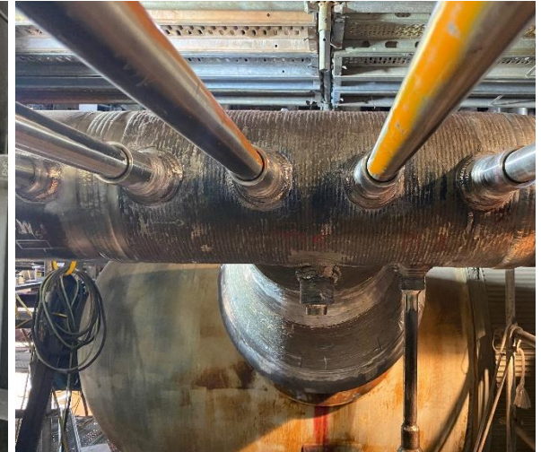
Piping components being printed at Lincoln Electric Additive Services
