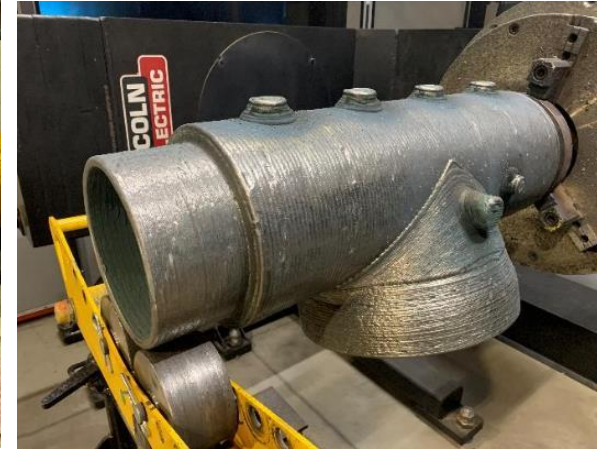
Piping components being printed at Lincoln Electric Additive Services
